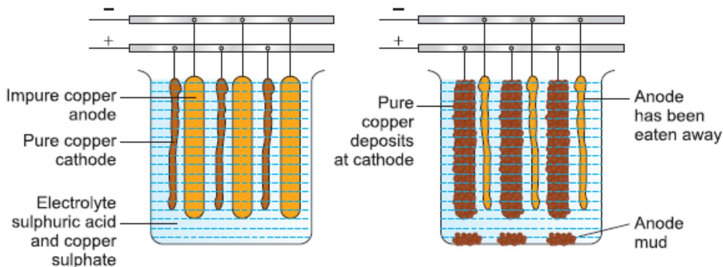
*Fig. 16.6 Electrorefining of copper.*
