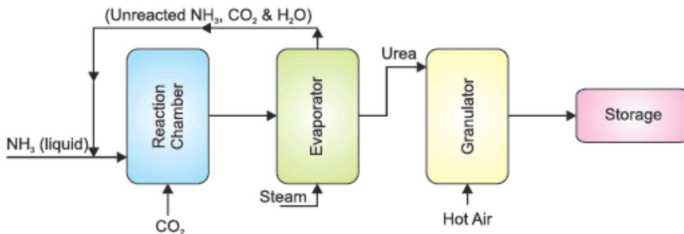
Fig. 16.9 Flow sheet diagram of Urea
