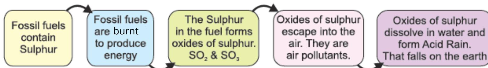
**Fig.14.6: Formation of SO<sub>3</sub> and SO<sub>2</sub> on combustion of fossils fuel and causing air pollution**
