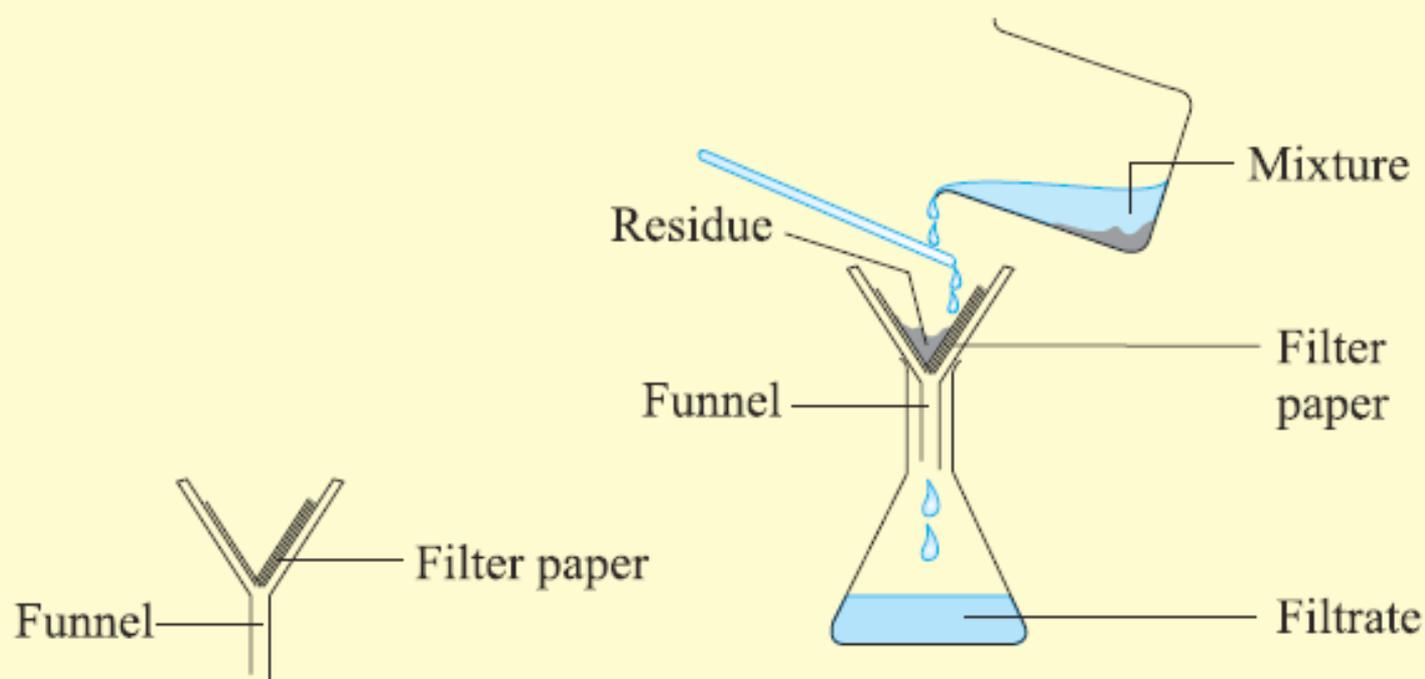
Filtrate passes through the filter paper and is collected in a conical flask. The solid particles (residue) deposit on the filter paper. It is then dried.
