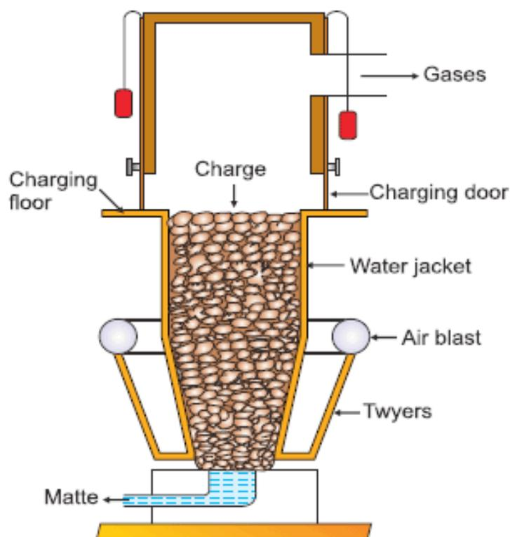
Fig. 16.4 Blast furnace for smelting of copper
