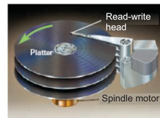
In computer hard drive, each platter has a magnetizable coating on each side. The spindle motor turns the platters at several thousand revolutions per minute (rpm). There is one read-write head on each surface of each platter.
