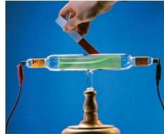
A cathode ray will deflect as shown when it is under the influence of an external magnetic field.
