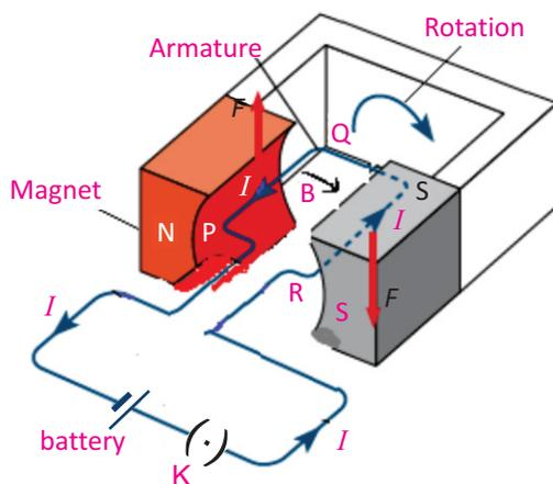
Fig. 15.8: A current-carrying coil in a magnetic field
