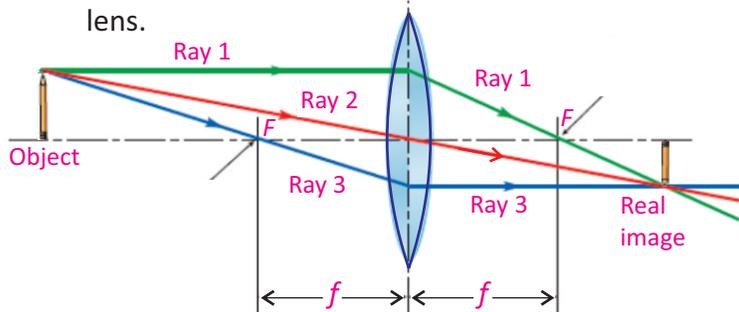
Fig. 12.23: Convex Lens
