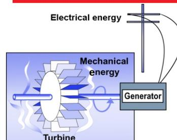
A generator inside a hydroelectric dam uses electromagnetic induction to convert mechanical energy of a spinning turbine into electrical energy.
