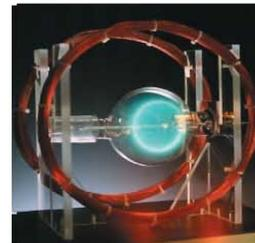
The glow in the tube is due to circular motion of electron in the magnetic field. The glow comes from the light emitted from the excitations of the gas atoms in the tube.
