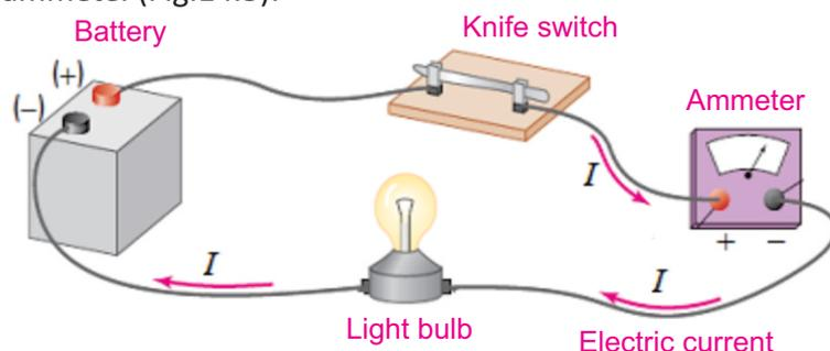
Fig.14.5: Schematic diagram showing the measurement of current
