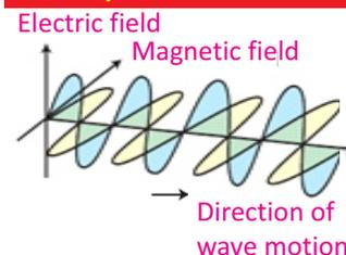
Electromagnetic waves consist of electric and magnetic fields oscillating perpendicular to each other.
