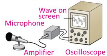
By using an oscilloscope, you can “see” sound waves.
