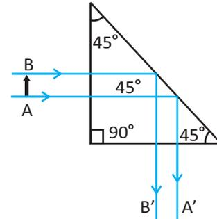
Fig.12.10: Total internal reflection through right angled prism
