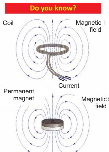
The magnetic field of a coil is identical to the field of a disk shaped permanent magnet.
