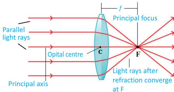
Fig. 12.20: Convex lens
