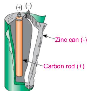
In a dry cell chemical energy changes into electric energy.
