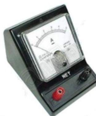
Fig.14.4: An ammeter
