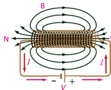
Fig. 15.4: Magnetic field due to a solenoid
