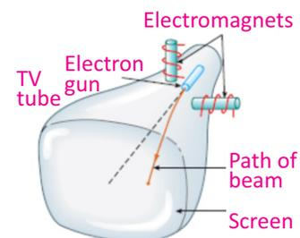
Electromagnets are used to deflect electrons to desired positions on the screen of a television tube.
