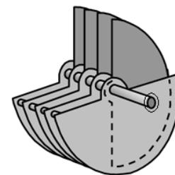
Fig. 13.19: Variable capacitor
