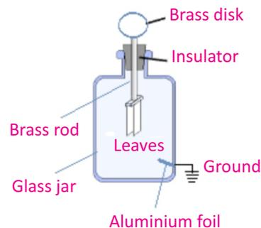
Fig.13.6: Uncharged electroscope
