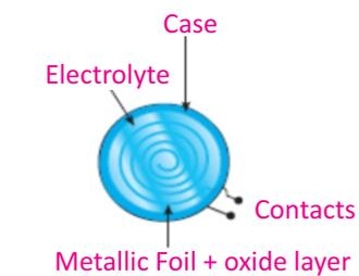
Fig.13.20: Electrolytic capacitor
