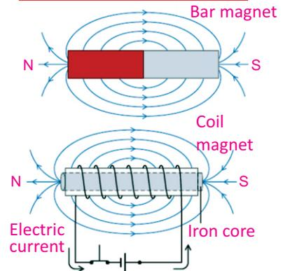
Similarity between magnetic fields of a bar magnet and that of a coil.
