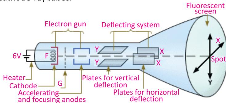
Fig. 16.4: Cathode-Ray Oscilloscope
