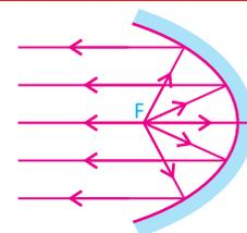
Parabolic mirror used in head lights.
