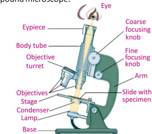
Fig.12.31: Compound microscope
