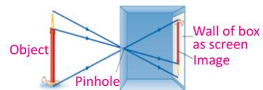
Even simpler than a camera with one lens is a pinhole camera. To make a pinhole camera, a tiny pinhole is made in one side of a box. An inverted, real image is formed on the opposite side of the box.
