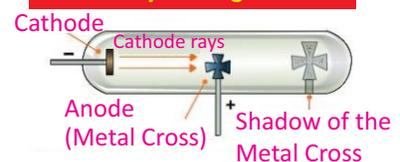
When an opaque object like a metal cross is placed in the path of cathode rays in a cathode-ray tube, a shadow of the metal cross is formed at the end opposite to the cathode. This is an evidence that rays of some kind are passing straight through the tube.
