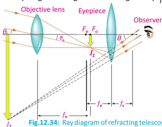
**Fig.12.34:** Ray diagram of refracting telescope
