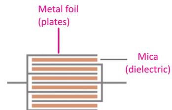
Fig. 13.17: Mica capacitor
