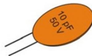
Fig. 13.18: Mica capacitor
