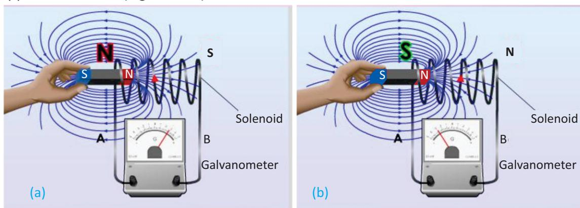
**Fig. 15.14:** Phenomenon of electromagnetic induction by the movement of a magnet through solenoid. (a) Magnet moves towards the stationary solenoid (b) Magnet moves away from the stationary solenoid
