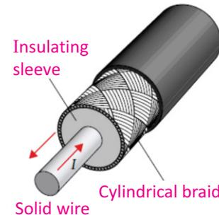
Coaxial cable wires are used to transmit electric signals such as cable TV to our homes. To prevent electric and magnetic interference from outside, a covering of conducting material surrounds the coaxial wires.
