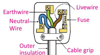
This is the correct way of wiring of a three pin main plug. Put everything in proper place. Fuse is placed for safety purpose. In case of excess current, it will burn out and will break the circuit.
