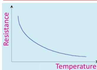
A thermistor is a temperature dependent resistor and its resistance decreases as temperature rises. Thermistor is used in a circuit that senses temperature change.
