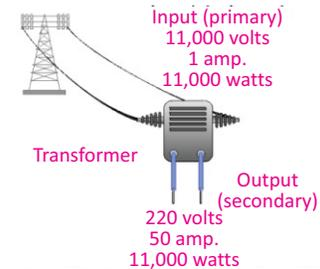
A high power transformer can reduce the voltage keeping the power constant.
