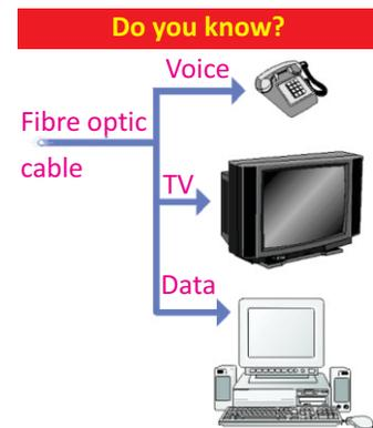
A single fibre optic cable can carry more than enough information to support television, telephone, and computer data.
