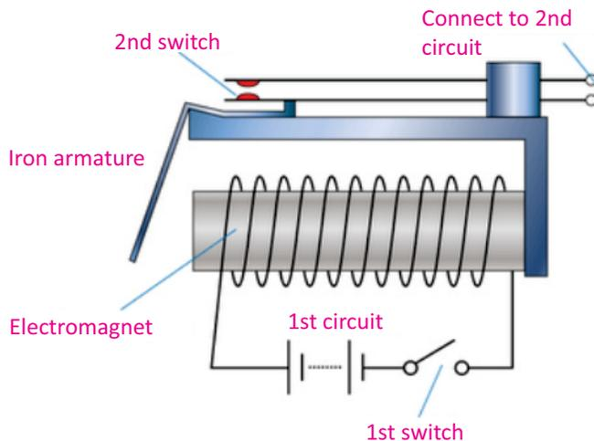
Fig. 15.21: Relay circuit
