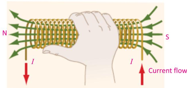
Fig. 15.5: Right hand grip rule for a coil
