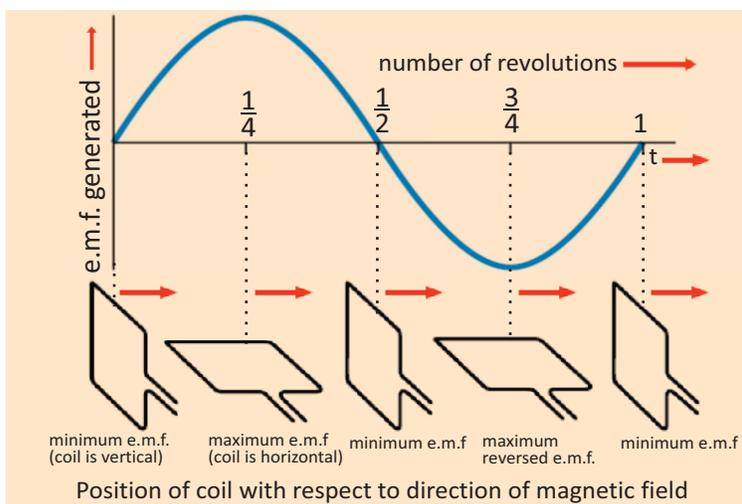
**Fig. 15.17:** e.m.f. Vs time for AC generator
