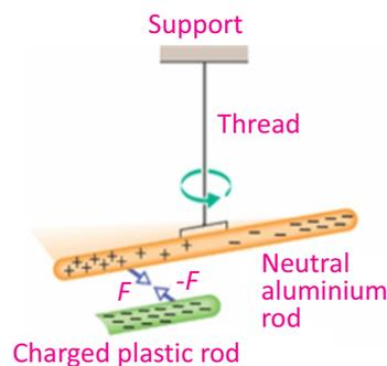
**Fig. 13.4:** Charged plastic rod attracts neutral aluminium rod.
