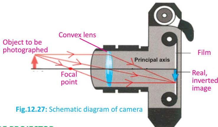
Fig.12.27: Schematic diagram of camera
