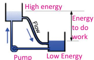
A battery raises electric charge back up to higher voltage (energy) just like a pump which pushes water back up to high energy so it can flow and do work again.
