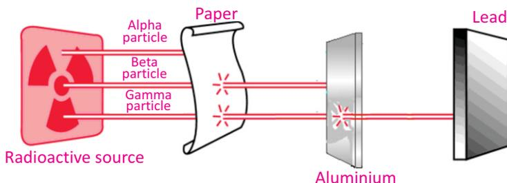
**Fig.18.6:** Penetrating power of radiations in different materials
